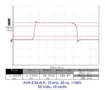
The AVR-E family offers medium-to-high voltage pulses with very fast rise and fall times.
